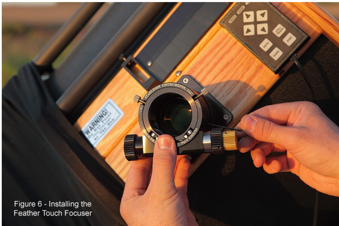
Figure 5 - Installing the Feather Touch focuser
